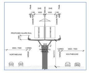
Figure 2 - 4 - Elevated Structure
