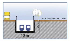
Figure 2 – 5 - Segregated Running in Retained Cut
